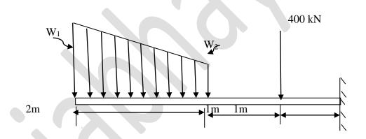
(c) For the beam shown in figure, taking the origin at A, find the equations for shear force and bending moment and draw SFD and BMD. The beam is subjected to a linearly varying load as shown in figure an A concentrated couple of 200kNm acts at 1m from end B.
