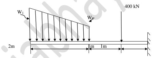
(c) For the beam shown in figure, taking the origin at A, find the equations for shear force and bending moment and draw SFD and BMD. The beam is subjected to a linearly varying load as shown in figure an A concentrated couple of 200kNm acts at 1m from end B.
